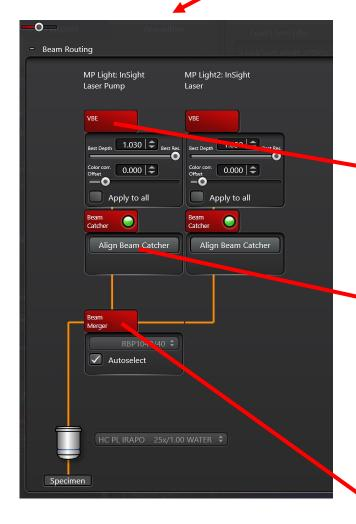
Set up the Variable beam expander. Using the beam expander, the diameter of the laser beam can be optimally adapted to the entrance pupil of the objective. It' a balance between depth and resolution.
