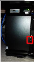
➤ IF it's not ON: Turn ON the Ti:Sapphire laser chiller (THIS IS HANDLED BY BIOVIS, IT SHOULD BE ON BY DEFAULT)
