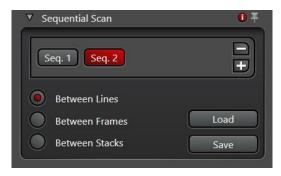
If sequential mode is activated, a new menu will pop up in the menus where the parameters of the sequential scanning can be configured. Here the excitation and emission settings for the different sequences (seq.1; seq.2, etc) can be checked and modified by clicking on any of the sequences.
