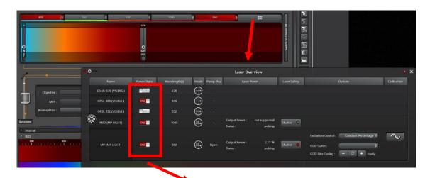
To turn OFF the lasers, use ONLY the ON-OFF sliders in the Laser Overview window (in the Acquire tab) or in the Laser Config window (in the Configuration tab).
