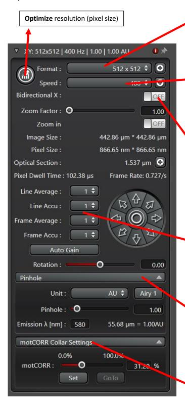
Set resolution (pixel size) manually. If you are unsure, use the **optimize** button. For 3D imaging use small, like 512x512 to save time/avoid bleaching.
