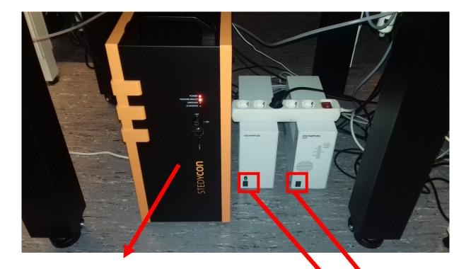
POWER STANDBY/READY EMISSION SCANNING The STEDYCON box is always on standby. When yellow light is visible next to the "Standby" text, follow the startup steps.
