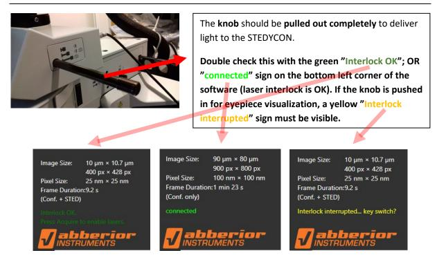
Don't go further and don't start any laser scanning if you see a problem with the laser interlock, as it can be dangerous! Never look into the eyepiece during laser scanning!
