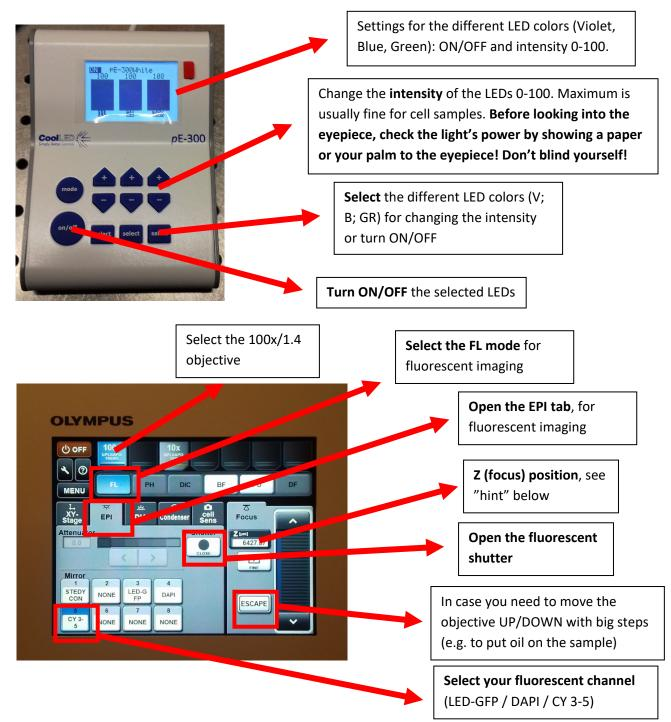
Now there should be light and fluorescent signal through the eyepiece. If nothing is visible, remember that there might be still no light to the eyepiece due to missed settings, malfunction, bad sample, or being in the wrong sample location (no cells in the field of view) etc... Don't start to move the objective UP/DOWN desperately, be careful.
