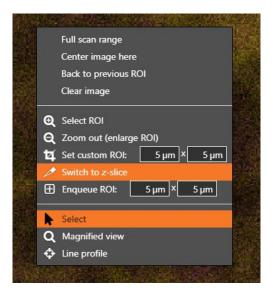
**Right-click** on the overview where Z-stacking is needed, and select the **"Switch to z-slice"** option.
