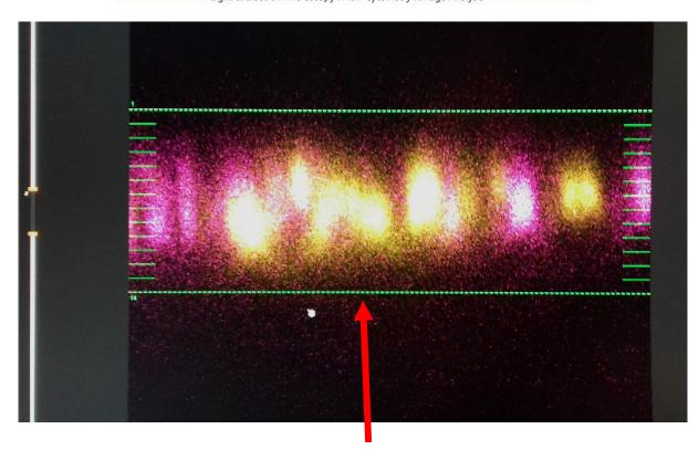
With left-click and holding the left mouse button, mark vertically the start (click left mouse button) and stop (release left mouse button) position for the Z-stack. The number of stacks will be visible on the screen. After this, hit the "Acquire button" and the 3D scanning starts in confocal AND/OR in STED mode.
