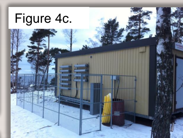
Figure 4c. Measuring station with resistive loads. (d) Wave measuring buoy 35 m from WEC. (e-f) Surveillance photos of WEC buoys surviving ice interaction.
