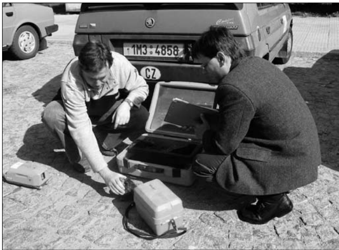
Figure 6.1 Preparation before an audit. The equipment is a laser for measuring gradient and alignment of pipelines. © KCM consulting.
