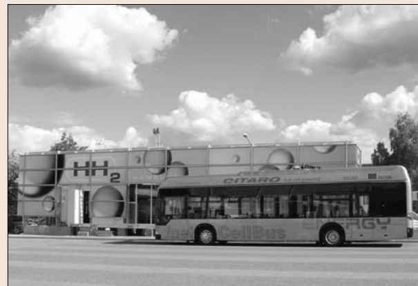
Figure 2.11 Bus with hydrogen-powered fuel cells in front of the fuelling station. Copyright © 2003 HOCHBAHN.
