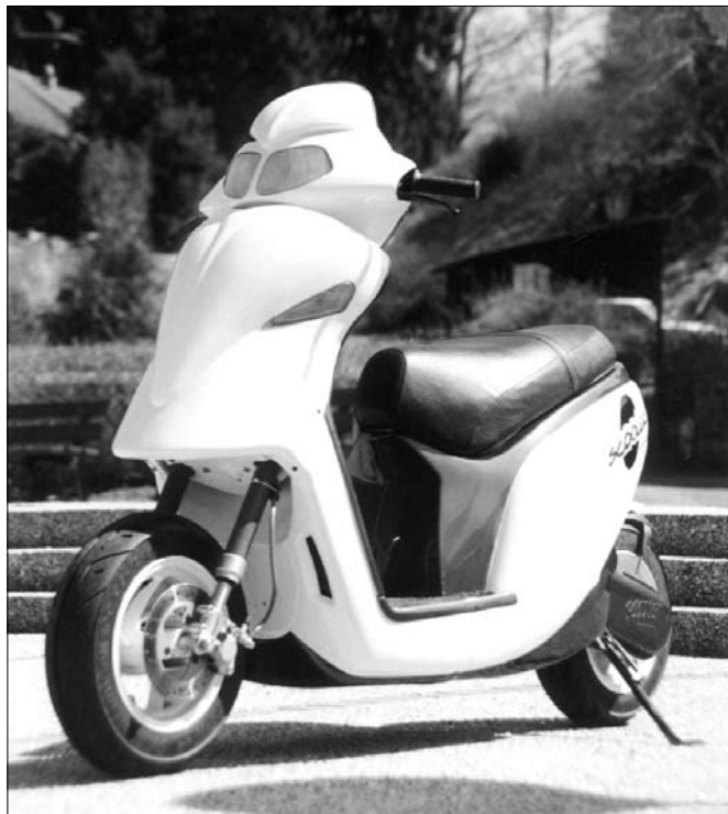
Figure 4.7 Electric scooter (Example 8). This scooter (the Scooler) runs on battery for 95 km on 45 km/h. Costs is about 10% of running a traditional gasoline motor scooter.
