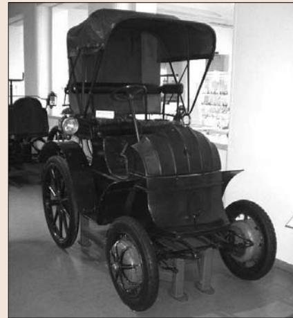
Figure 2.7 The Lohner-Porsche. The electric engine was placed in the front hubs. (The Lohner-Porsche Electric-Car is part of the Exhibitions of the Technisches Museum Wien.)
