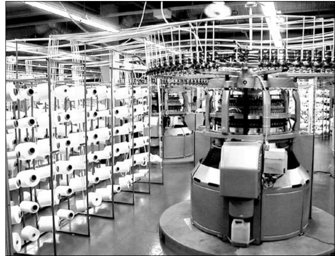
Figure 1.2 Production starts with the yarn, which is knitted in the knitting department at a capacity of 2,000 to 2,300 kg a day.
