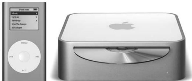
Figure 4.13 Mini MP3-player and computer (Example 17). The Apple iPod and Mac mini computer illustrate a dramatic case of dematerialisation. Despite their compact design, they are equipped with large hard disks and many other functions
