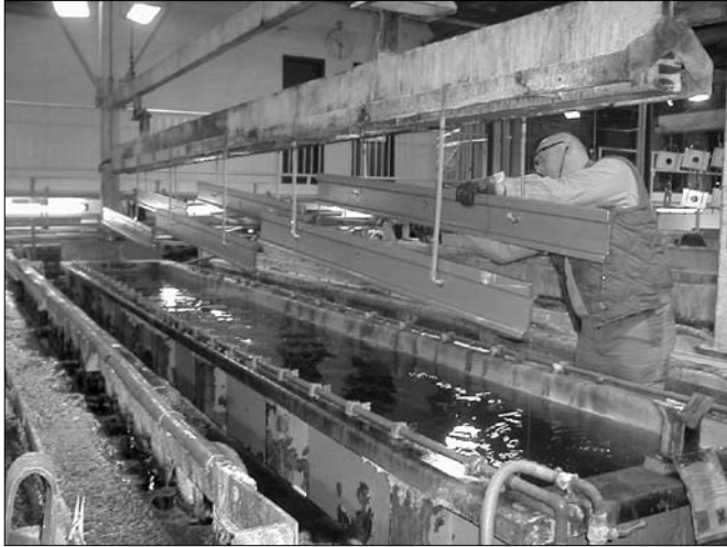
Figure 6.1 Rinsing bath. Last rinsing before going to the bath for the electroplating, i.e. being covered by a thin layer of zinc. You see 'spray-rinsing' instead of dipping the whole item in the bath. Means less polluted water in the process. (Photo: Roskilde Municipality Environmental Inspection office)
