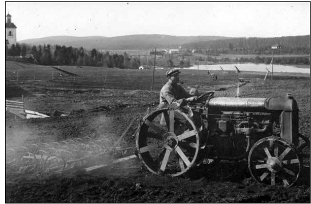
Figure 7.6. Fuel-powered agriculture represented by this Fordson tractor produced by Henry Ford between 1916-1928. The Fordson Model F was the first small, mass-produced and affordable tractor in the world. In Ford signed an export contract with the Soviet Union for which soon became the most important customer of the company. In 1924, the "Red Putilovite" factory in Leningrad started the production of Fordson-Putilovets tractors. These inexpensive and robust tractors became an important enticement for peasants towards collectivisation and were often to be seen on propaganda posters and paintings. Photo: Unknown. Probably 1930s in Hälsingland, Sweden. Source: Sockenbilder.
