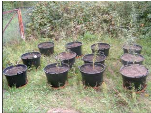
Figure 17.3. Treatment of municipal wastewater treatment plant effluent in soil-willow system experiment. Results show high removal of phosphorus and medium removal of nitrogen from wastewater (see above). Photo: Agnieszka Karczmarczyk
