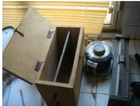
Figure 27 Wood box with heater inside. Coil and resistor
