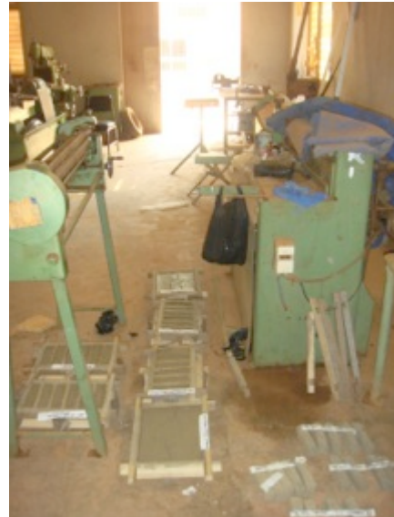
Figure 24 The samples were protected against rain, wind and sun during drying but the conditions could not completely be controlled
