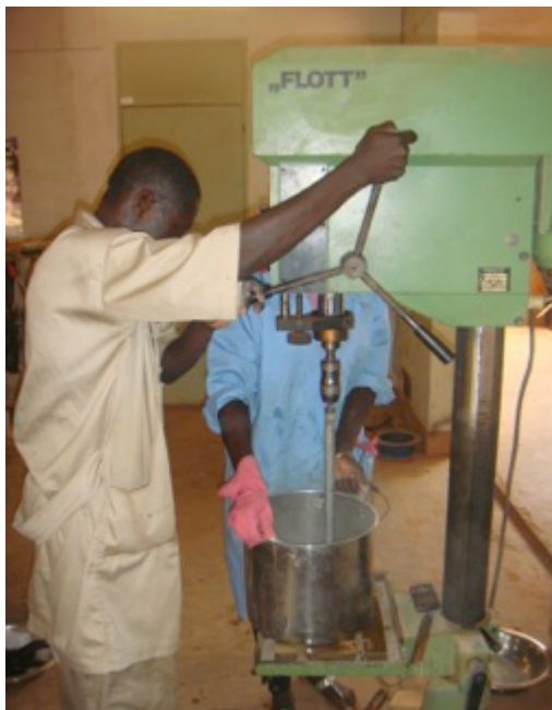
Figure 23 The materials were mixed with a power drill and then casted in a mold for vibration
