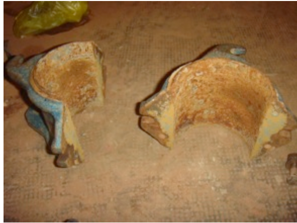
Figure 32 Corrosion on the metal molds
