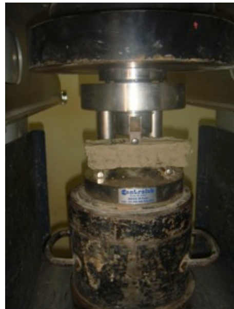
Figure 29 Device for measuring tensile strength
